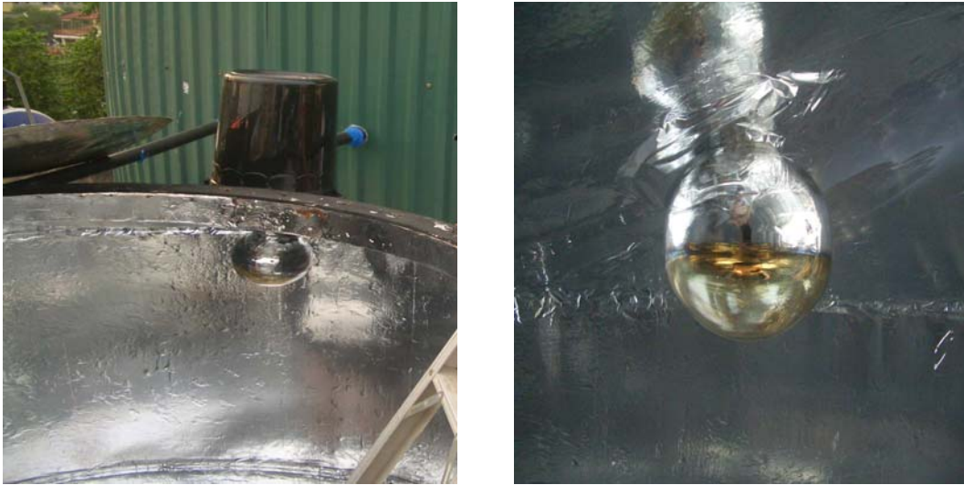
Figure 2.17 Photonis PMTs have been installed in the main VATLY Cherenkov Counter
