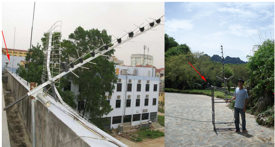
Figure 5.4 Antenna mountings. Left: early flagpole mounting on the roof of our laboratory. Right: equatorial mounting in Hoa Binh. The arrows indicate the second antenna.
