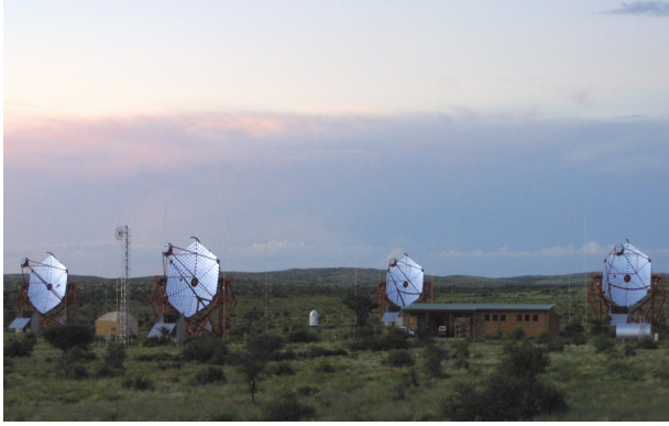
Figure 6: The High Energy Stereoscopic System (HESS, Namibia) includes four telescopes at the corners of a 120 \times 120 \text{ m}^2 square, operating above 100 GeV. Its field of view is 5^\circ and its resolution a few arc minutes. To take a picture of the Crab takes only 30 seconds.
