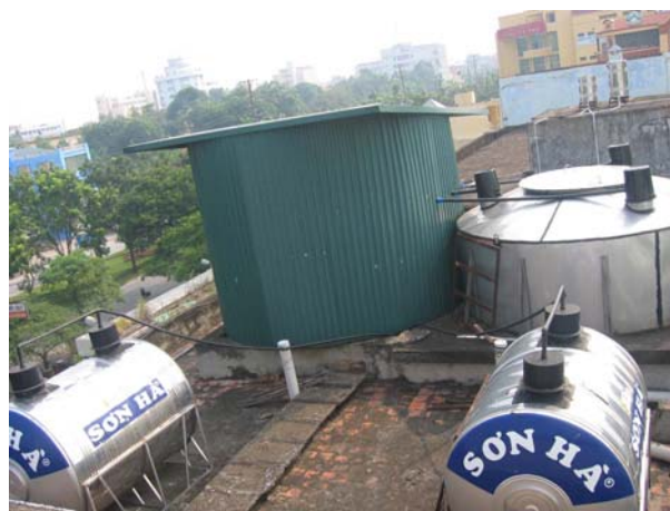
On the roof of the laboratory: the large Auger tank on the right and two of the three trigger tanks (the third one is hidden behind the hut)
