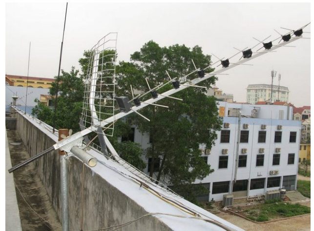
One of the interferometer antennas on the roof of the laboratory
