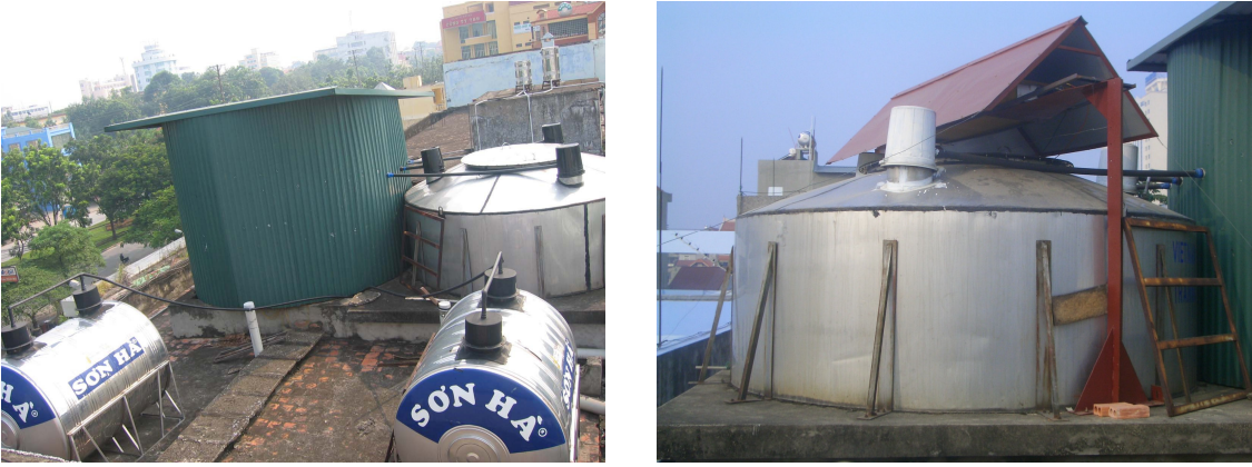
Figure 1.13 Left: The main Cherenkov detector is seen surrounded by two of the three smaller ones, one of which is hidden behind the green tower. Right: Addition of a scintillator hodoscope to the main Cherenkov detector; the lower part of the hodoscope is located in the counting room below the roof.
